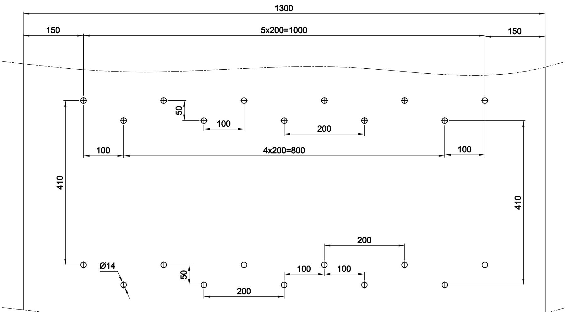
Punching drawing of the elevator belt for project no. 42416
